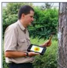
The ARBOTOM® is a novel impulse tomography unit that enables an inside view of condition of trees and round wood. Hidden decay, invisible cavities and cracks and how large they are become visible with ARBOTOM® using sound impulses.
